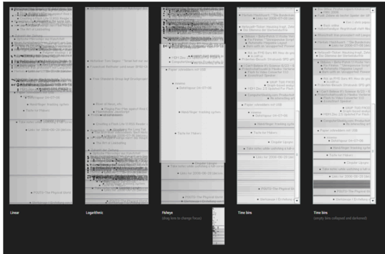
Figure 45: Different approaches to time visualization (Left to right: linear, logarithmic, fisheye distortion, time bins, time bins with gap indication)
